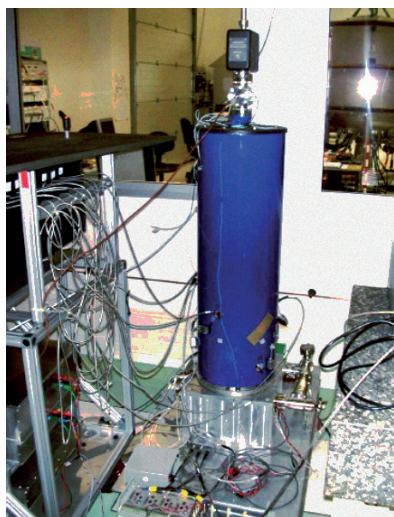
Figure 8: The transportable caesium fountain FOM of LNE-SYRTE at the Toulouse laboratory of CNES (Centre National d'Etudes Spatiales, France) in preparation of the ACES mission. (Courtesy of LNE- SYRTE, Paris)
