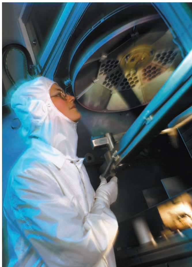
Figure 4: Precise control of light states requires the use of high-end technologies in experimental setups. Special optical components and coatings are designed and fabricated within the framework of QUEST as shown in this picture of the coating facility at LZH (courtesy of LZH).
