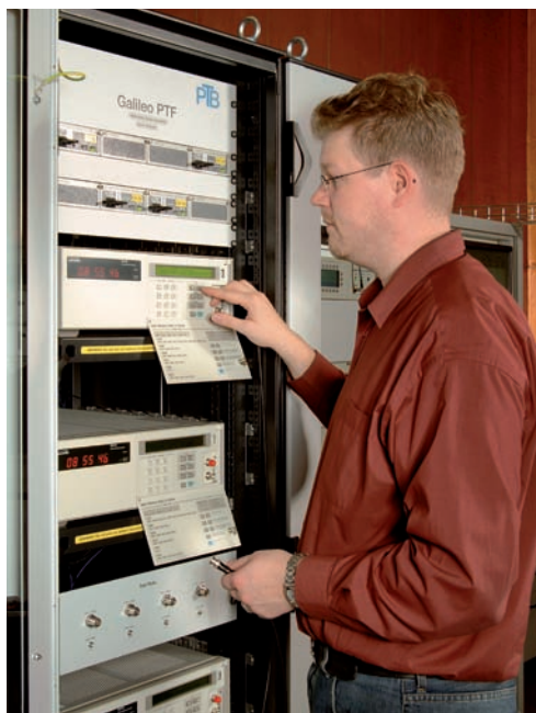
Figure 5: The contribution of PTB to the Galileo Ground Segment instrumentation: Michael Rost making final adjustments to the ground caesium clocks. The rack to the right contains the Galileo System Time realization subsystem. Work performed under contract with Kayser-Threde GmbH, Munich, Germany.
