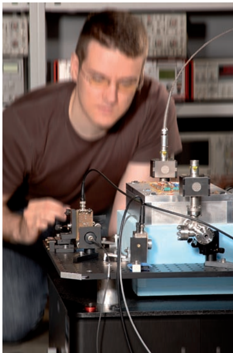
Figure 4: Vibration isolation (digitally edited photo). The reference cavity is mounted on a passive vibration isolation platform (lower right). The vacuum vessel containing the reference cavity is held in a massive temperature-stabilized aluminium box. Thermal isolation material (light blue) has been partly removed. The optical setup on the platform comprises the Pound-Drever-Hall frequency discriminator and optics for fiber coupling and mode matching.
